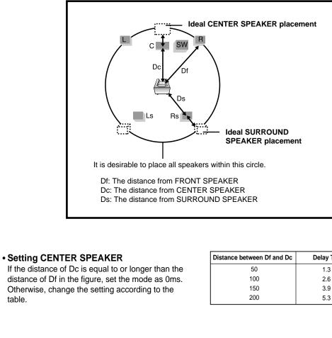
• Setting REAR (SURROUND) SPEAKERS If the distance of Df is equal to the distance of Ds in the figure, set the mode as 0ms. Otherwise,
